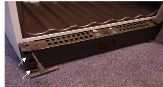
6. Dismount 4mm Allen screws and remove the column. Hereafter, the base plate can be dismantled from the cabinet.
